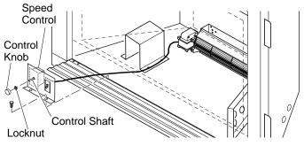
Figure 32 - Attaching Speed Control to Firebox
